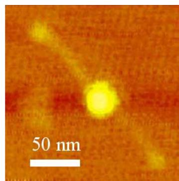
**Figure 4.** nc-mode AFM image using standard Pt/Ir coated tip. The DNA shown had an apparent FWHM of 11 nm.
