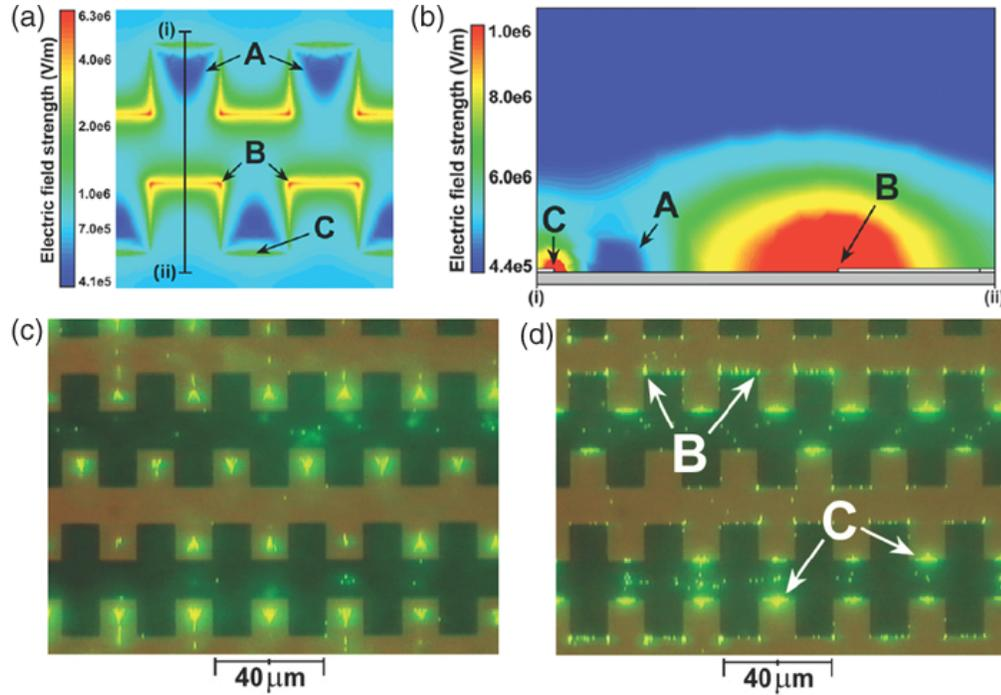
Figure 3.6: Positive and negative DEP for latex spheres, from Green *et al.* (2000). (a) Numerically-calculated electric field 100 nm above castellated electrodes. (b) Electric field in the vertical slice between points (i) and (ii) in (a). (c) Negative DEP is observed for 557-nm latex spheres when the applied signal is 8 volts peak-to-peak at 8 MHz. (d) When the field frequency is reduced to 700 kHz, positive DEP occurs.
