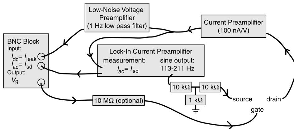
Figure 6.9: Electrical measurement setup. An AC or DC bias voltage,  $V_{sd} = 5\text{--}50\text{ mV}$ , was applied to the source while a LabVIEW program was used to sweep the gate voltage  $V_g$  and to measure the current  $I_{sd}$  passing through the drain. AC measurements also enabled simultaneous measurement of the leakage current  $I_{leak}$  between the gate and the drain.
