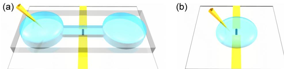
Figure 9.3: Measurement schematic for *Dictyostelium* measurements. The cells in buffer were either (a) placed in a PDMS channel that was sealed over the nanotube device or (b) placed directly over the nanotube with no PDMS.
