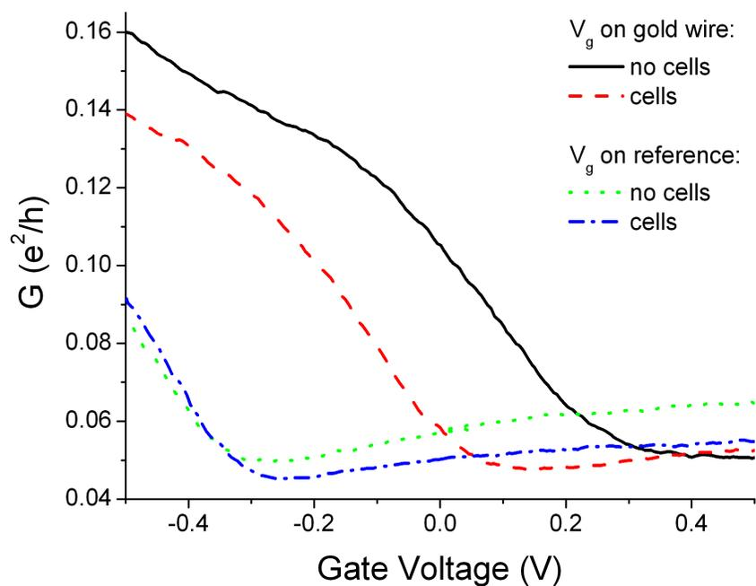
Figure 9.5: Conductance vs. gate voltage when *Dictyostelium* is added to a PDMS channel with a nanotube. The threshold voltage shift observed when the gate voltage is applied to a gold wire disappears when a Ag/AgCl reference electrode is used instead. The background solution was phosphate buffer.
