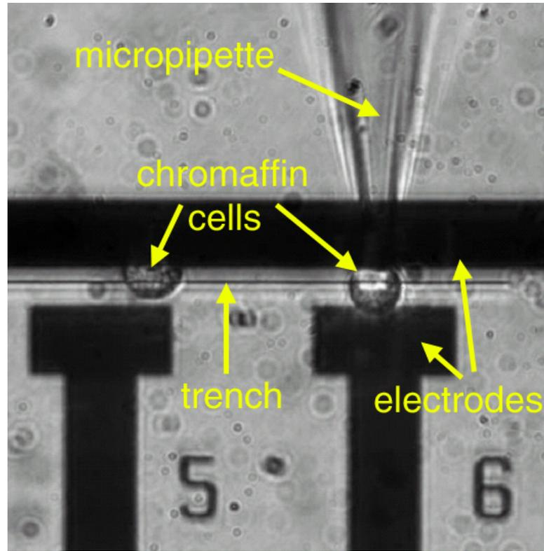
Figure 9.7: Brightfield image of a chromaffin cell over a suspended nanotube. The spacing between the source and drain electrodes is  $10 \mu\text{m}$ . A micropipette is seen holding a cell over device 6, while a second cell is seen over device 5. The other smaller circles are dust in the microscope optics.
