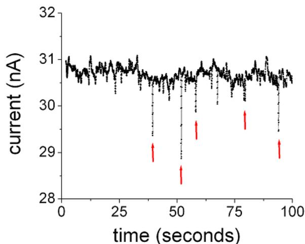
Figure 8.4: Second example of electrical response of nanotube to DNA. In this experiment (in which  $V_{sd} = 10$  mV), five of the initial spikes (marked with red arrows) were correlated with a dsM13 DNA molecule passing the nanotube, but subsequent spikes were uncorrelated.
