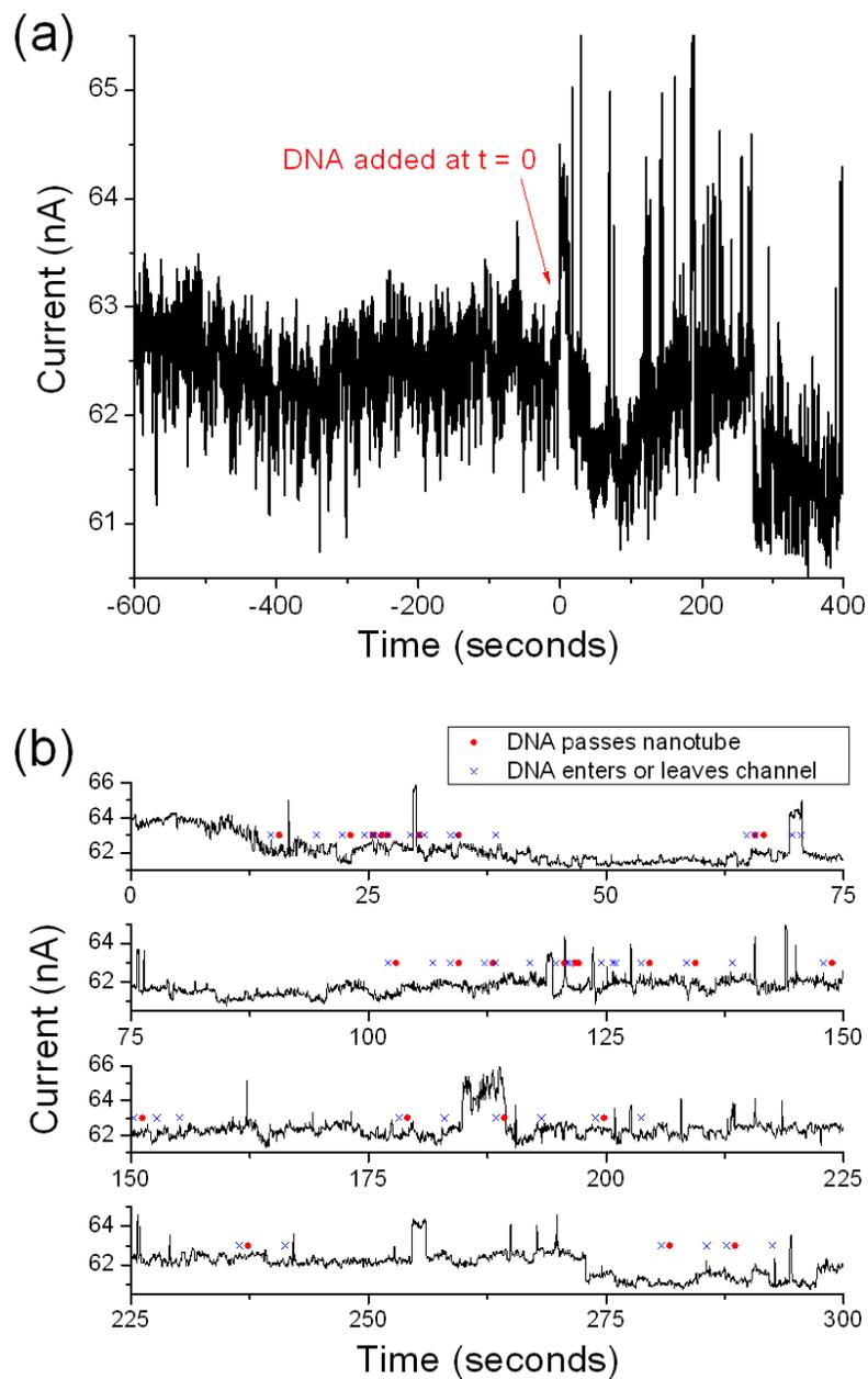
Figure 8.3: Electrical response of nanotube to DNA, with  $V_{sd} = 10$  mV. (a) The nanotube current showed much more fluctuation after the introduction of dsM13 DNA to the PDMS channel. (b) Although the initial current spike occurred at roughly the same time as the first DNA molecule passed the nanotube, subsequent spikes were uncorrelated.
