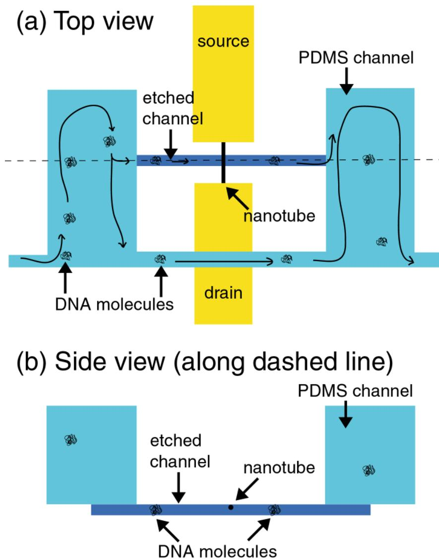
Figure 8.1: Schematic of microfluidic system for bringing DNA to a suspended nanotube. (a) Top view. A narrow channel is etched under the nanotube in the  $\text{SiO}_2$  surface, and a larger PDMS channel is used to bring DNA molecules into this smaller etched channel. (b) Side view of the microfluidic setup along the dashed line in (a).
