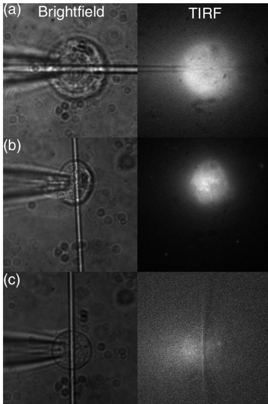
Figure 9.14: Brightfield and TIRF imaging of a cell over a 1- $\mu\text{m}$ -wide trench. The three images on the left are brightfield pictures of a chromaffin cell held by a micropipette over a trench, and the three images on the right show the same cells imaged with TIRF microscopy. Cells (a) and (b) were dyed with DiIC<sub>18</sub>(3), and cell (c) was dyed with FM1-43. Cells were dyed and imaged by Kassandra Kisler.
