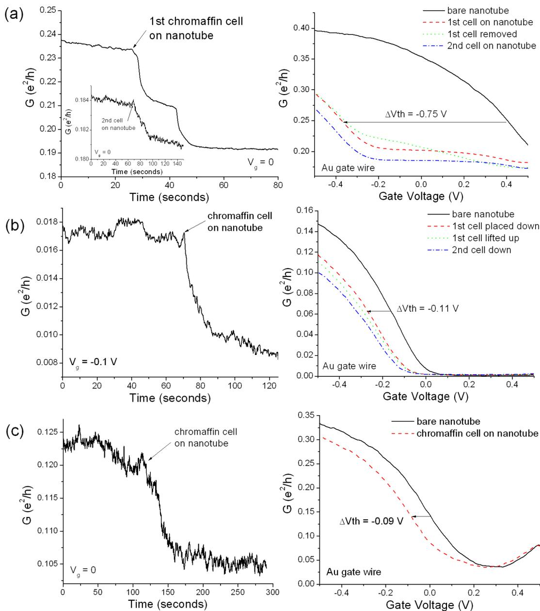
Figure 9.9: Response of suspended nanotubes to chromaffin cells.  $G$  vs.  $t$  and  $G$  vs.  $V_g$  are shown for three different nanotube devices, all of which show a negative threshold voltage shift after a cell is placed on top of them.
