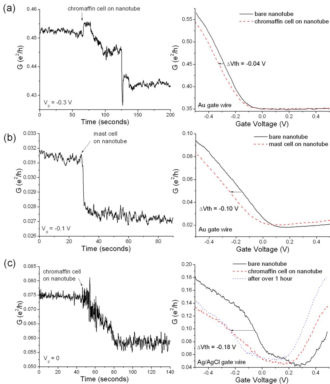
Figure 9.10: Response of suspended nanotubes to chromaffin and mast cells. As in Figure 9.9,  $G$  vs.  $t$  and  $G$  vs.  $V_g$  are shown for different nanotube devices, which show a negative threshold voltage shift after a cell is placed on top of them.
