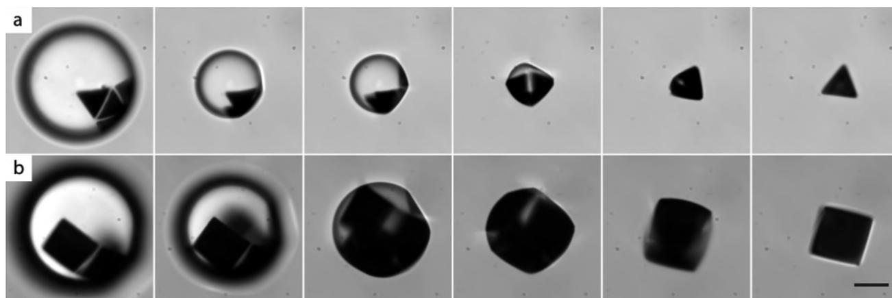
**Figure 3.** Self-folding with chloroform droplets. Image time series of self-folding of a, a tetrahedron, and b, a cube, with droplets of chloroform. Since chloroform is partially miscible in water, the shapes fold as the chloroform dissolves into the water. The scale bar is  $25\ \mu\text{m}$  long. Videos of these shapes can be found in [Supporting Video 4](#).
