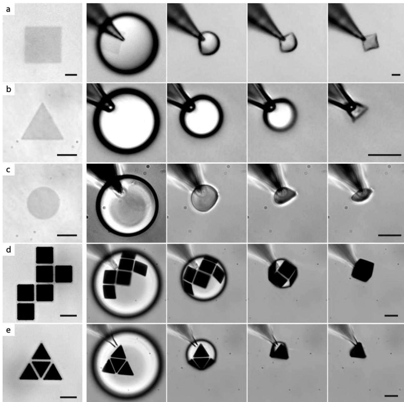
**Figure 2.** Image time series of the folding of both MoS<sub>2</sub> shapes and shape nets. The leftmost figure in each row shows the initial, unfolded shape. a–c, Square, triangular, and circular sheets folding into square, tetrahedron, and “empanada” packets, respectively. d,e, folding of shape nets (Cu panels and MoS<sub>2</sub> hinges) into a cube and a tetrahedron. All scale bars are 20 μm long. Videos of these folding shapes can be found in [Supporting Video 1](#).
