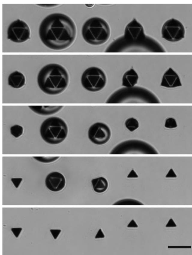
**Figure 4.** Parallel folding of shapes using chloroform emulsions. A microemulsion of chloroform was added to unreleased shape nets. Diluted hydrofluoric acid was then added to the solution so that the final ratio of hydrofluoric acid to water was approximately 1:50. Folding took place over about 15 min. The scale bar is  $50\ \mu\text{m}$  long. Video of this parallel self-folding can be found in [Supporting Video 5](#).
