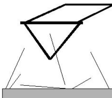
**Figure 2.** Schematic diagram of pick-and-stick procedure for mounting CNT tip onto cantilever.
