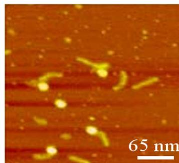
**Figure 3.** An nc-AFM image of RNAP–DNA complexes scanned with a silicon tip of approximately 10–20 nm diameter. It shows tip–surface interaction effects such as the polymerase complex depicted as featureless white spheres and the DNA strands as rodlike fragments. The indicated dimensions of the polymerase and the DNA strands have also been enlarged by the tip–surface interaction.
