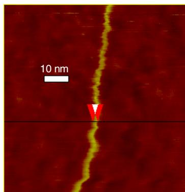
**Figure 1.** Nanotube imaged with a nanotube AFM tip showing high resolution and mechanical noise from the AFM instrument. The AFM instrument used in this image was the Digital Instruments Dimensions AFM mounted on a floating optical table. The height of the tube is 1.3 nm and the full width at half maximum is 2.75 nm so the effective AFM tip radius assuming a two-sphere model is 1.29 nm. All images were processed with a flattening filter.
